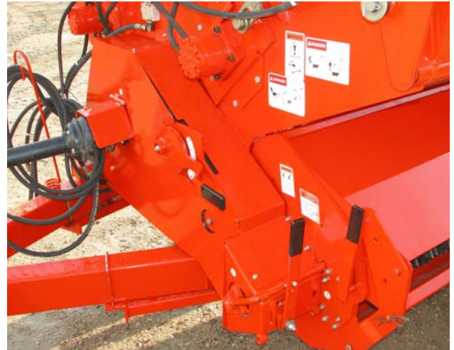
Ensure All Drive Shields Are In Place
