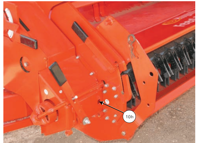
Grease Front Rotor Bearing
