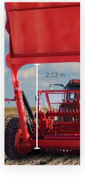
The High-Lift design feature provides options for operators to get rocks out of the way or off the field. The High-Lift minimizes wasted space from low flat rock piles by allowing higher more compact piles , or rocks can be transferred directly to a trailer for removal. For fast and convenient rock removal, Highline<sup>®</sup> NT60E rock pickers have a standard dumping height of 2,13 m.
